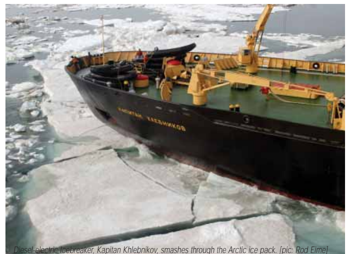
Diesel-electric icebreaker, Kapitän Khlebnikov, smashes through the Arctic ice pack. [pic: Rod Eime]
